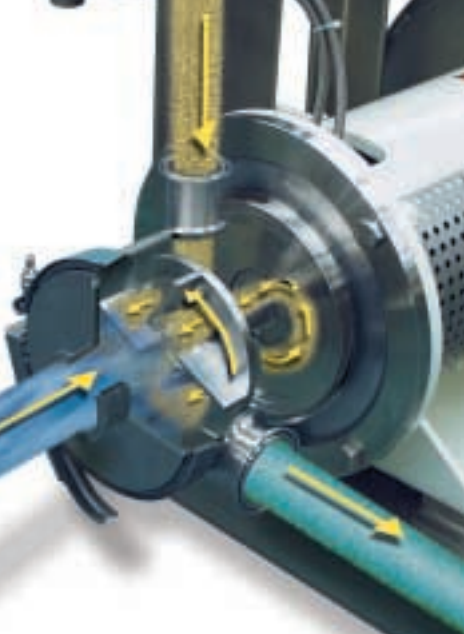
The rotor/stator generator in the SLIM system draws a large volume of powder (shown in yellow) into the high shear zone, where it is simultaneously combined and mixed with the liquid stream (blue).
