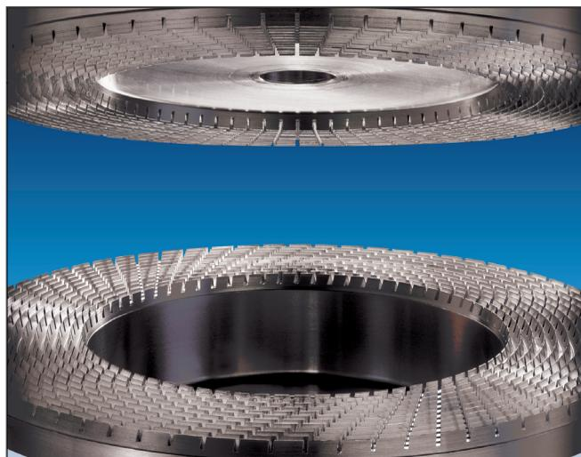
**FIGURE 6.** The rotor and stator of an ultra-high shear mixer (UHSM) are made up of many concentric rows of intermeshing teeth. The rotor turns at extremely high speed — reaching tip speeds as high as 18,000 ft/min. Fluid begins at the center of the generator and moves outward through radial channels cut in the rotor/stator teeth. As the mix material moves toward the outlet, it is subjected to intense mechanical and hydraulic shear — and thousands of shearing events in each pass
