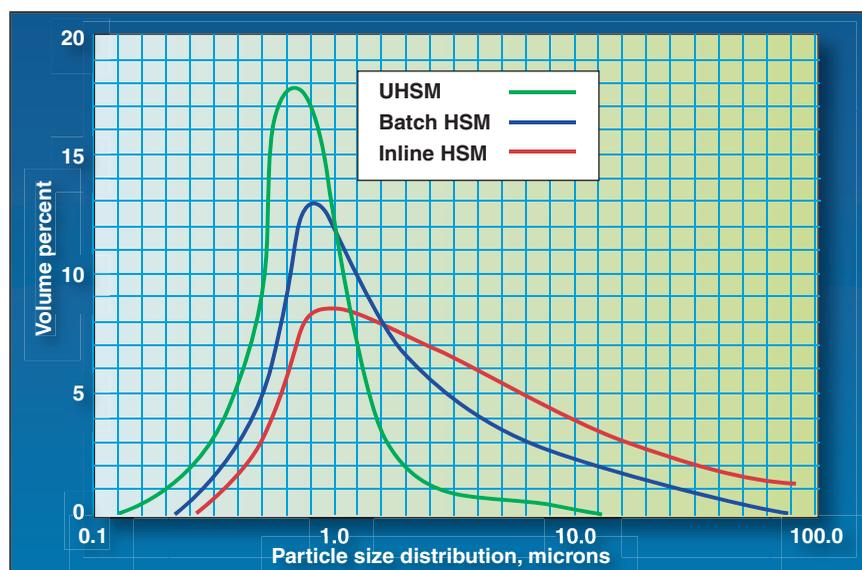
**FIGURE 7.** Shown here are the particle-size distributions one can expect to achieve with a batch HSM, inline HSM and UHSM. Both the batch and inline HSMs shown here are 10-hp units operating with a 100-gallon tank, recirculating for the required four minutes. In applications where a narrow particle-size distribution is required — signifying an extremely uniform emulsion or dispersion — the UHSM should always be evaluated as a potentially cost-efficient design alternative
