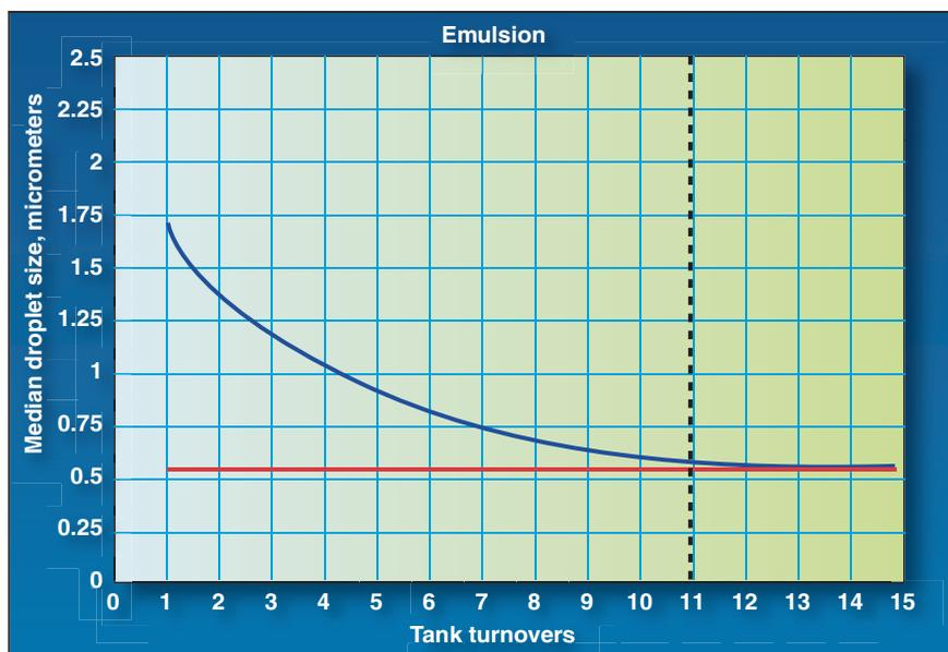
**FIGURE 4.** This graph shows the mixing equilibrium curves for a typical emulsion. The horizontal line represents the asymptote; the vertical line represents the equilibrium point. During high-shear mixing, the desired characteristic is reached in a given amount of time. Beyond this point, additional mixing will just result in wasted effort, energy and wear and tear on the equipment
